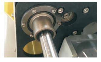
4 Spline gearing device
